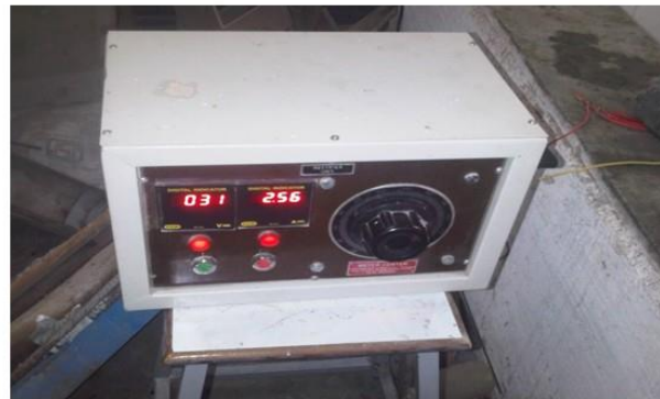
Figure 6: Rectifier for DC power supply
