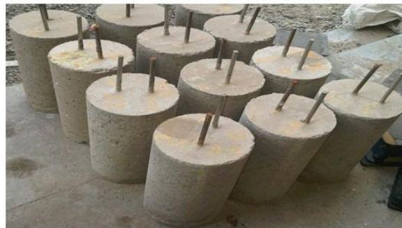
Figure 3: Specimens for accelerated corrosion test
